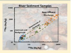
Marcellus Shale produced waters. Nonetheless,  ${}^{226}$ Ra levels in stream sediments (544–8759 Bq/kg) at the point of discharge were ~200 times greater than upstream and background sediments (22–44 Bq/kg) and above radioactive waste disposal threshold regulations, posing potential environmental risks of radium bioaccumulation in localized areas of shale gas wastewater disposal.
